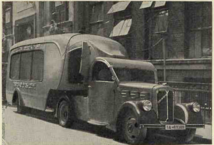
A large van equipped with the Loewe transmitting and receiving apparatus was brought to London for the purpose of the demonstration. Transmission was made upon 7 metres to a receiver in the annexe of the Polytechnic.
