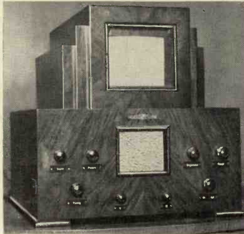
A view of the Loewe 180-line television receiver which it is stated could be marketed for about £30.
