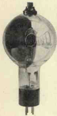
A photo-cell intended for television and other purposes where only small illumination is available. This is the X41 made by the Oxford Instrument Co., and at one metre from a 40 watt lamp the vacuum type gives an output of 10 micro-amps.
