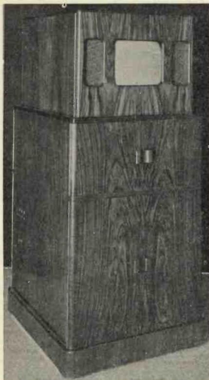
The Fernseh A.G. 180-line cathode-ray receiver, a new German apparatus which is reported to give very fine results.
