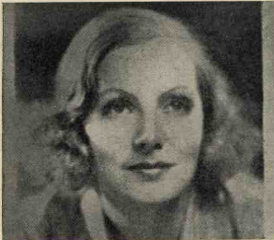
Left—The definition obtainable of a single face with a scanning frequency of 120 lines. On the right is a small group, also of 120-line definition.
